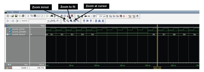
Click on the waveform put a cursor at a specific time for inspecting the signal values.
